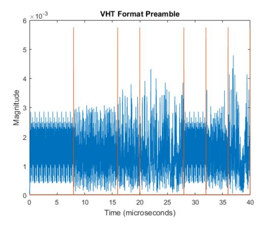
Demodulate the L-LTF and estimate the channel.
