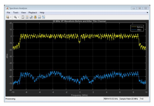
Path loss accounts for the roughly 50 to 60 dB of separation between the waveform before and after it passes through the TGn channel. The path loss results from the default transmitter-to-receiver distance of 3 meters, and from shadowing effects. The signal level variation shows the frequency selectivity of the delay profile across the frequency spectrum.
