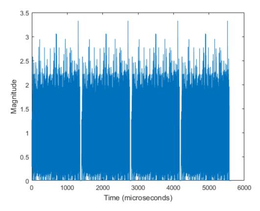
The plot shows four non-HT format OFDM modulated packets, with  $45\ \mathrm{microseconds}$  of idle time separating each packet.
