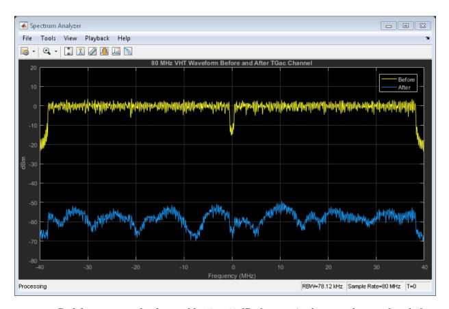
Path loss accounts for the roughly 50 to 60 dB of separation between the waveform before and after it passes through the TGac channel. The path loss results from the default transmitter-to-receiver distance of 3 meters, and from shadowing effects. The signal level variation shows the frequency selectivity of the delay profile across the frequency spectrum.
